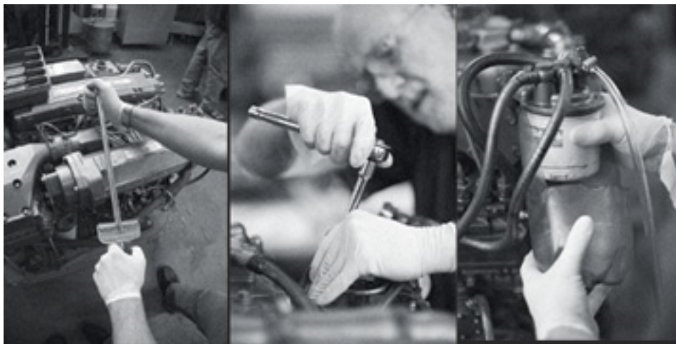
Reading a torque wrench (left), disassembling heat exchangers (middle), and changing fuel filters (right) are some of the classroom topics.
