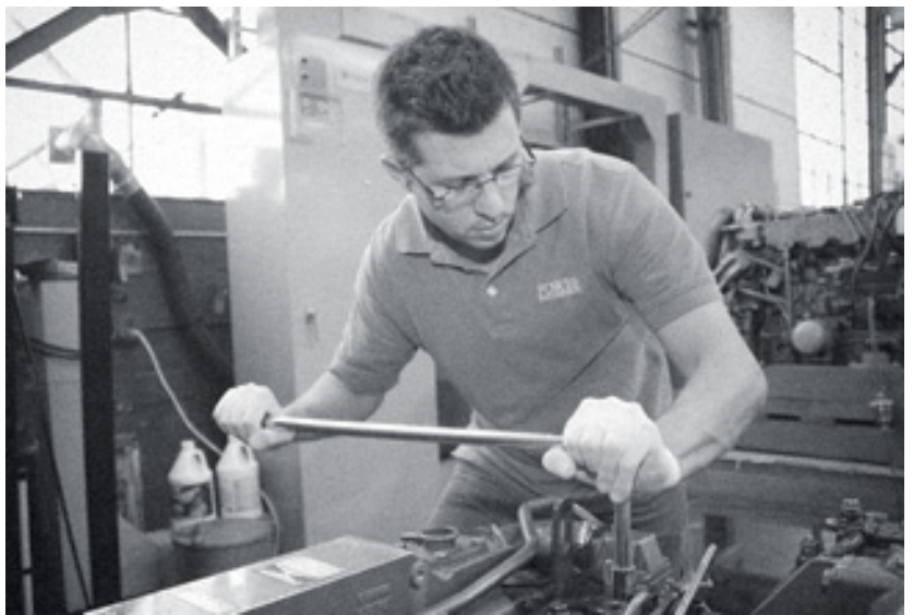
Loosening the cylinder-head bolts requires a long wrench and some good ol' muscle.
